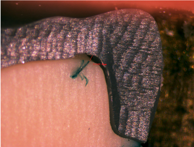
Figure 6. Representative image of measurements taken with the stereomicroscope. This example is of a Dentsply wax showing a 152.05µm gap between wax and printed die.
